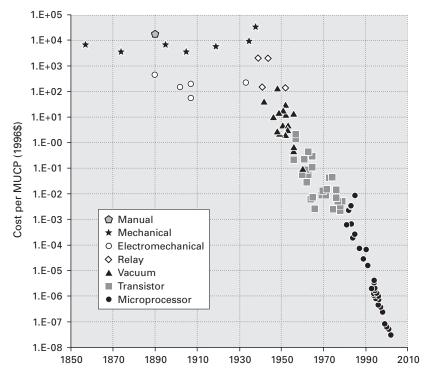
**Figure 1.2** Increasing cost efficiencies of computation with a marked step change from mechanical to electronic processing technologies. (Redrawn from Nordhaus 2002, 43)
