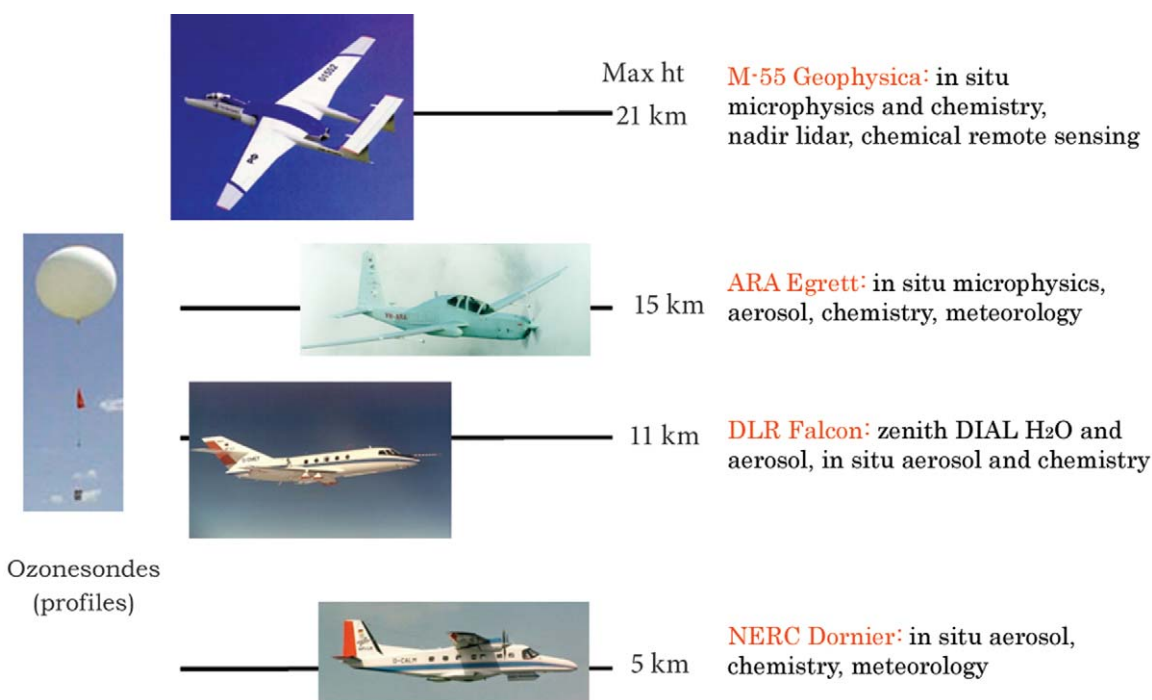
FIG. 1. Montage showing the aircraft used in the campaign, with a brief description of their function and altitudes of operation.
