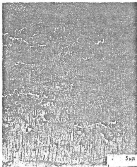
4 Section through a porous anodic film on aluminium.
