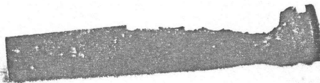
3 Severe hot corrosion of a gas turbine stator blade.
