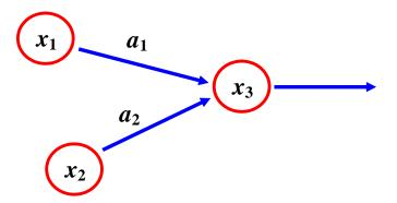
$$\begin{array}{rcl} x_3 & = & \max\left(x_1 + a_1, x_2 + a_2\right) \\ & = & a_1 \otimes x_1 \oplus a_2 \otimes x_2 = (a_1, a_2) \otimes \left(\begin{array}{c} x_1 \\ x_2 \end{array}\right) \end{array}$$
